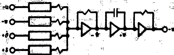
Figure VIII-7. Mechanization of the \dot{w} equation
