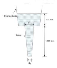
Considering the cross-section of the sprue is circular, the ratio d<sub>1</sub>:d<sub>2</sub> to avoid aspiration is
