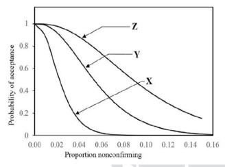
Considering the above operating characteristic curves, the correct relationship of the plans with respect to sample size is
