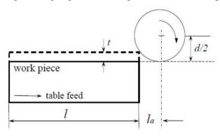
If t is the depth of cut and d is the diameter of the milling cutter, then the length of approach  $(l_a)$  is expressed as
