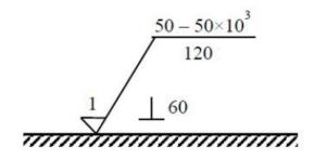
The waviness height (in micrometer) of the surface is
