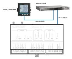
Figure 7-7 AcuLink 810 Modbus TCP Connection
