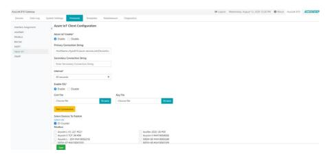
Figure 7-50 AcuLink 810 Azure IoT Client Configuration
