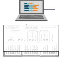
Figure 4-1 AcuLink 810 Ethernet Direct Connection to PC
