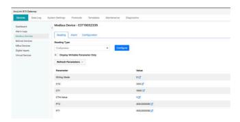
Figure 8-12 AcuLink 810 Reading Modbus Register Values After Change
