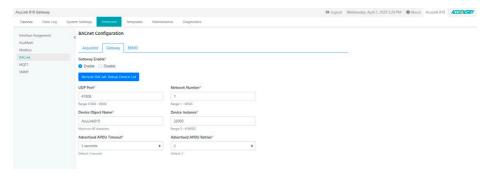
Figure 7-42 AcuLink 810 BACnet Gateway Function Setting
