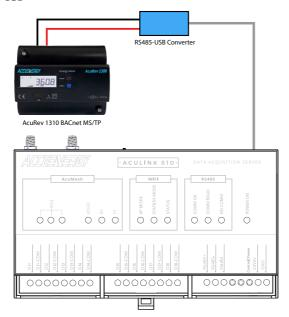
Figure 7-31 AcuLink 810 BACnet MS/TP via RS485 to USB Converter
