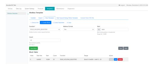
Figure 5-5 AcuLink 810 Saved Modbus Templates
