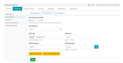
Figure 10-5 Post Channels SFTP Configuration
