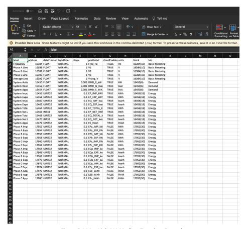
Figure 5-14 AcuLink 810 Modbus Template Example
