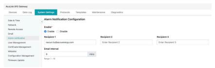
Figure 9-11 AcuLink 810 Alarm Notification Configuration
