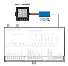
Figure 7-2 AcuLink 810 Modbus RTU Connection
