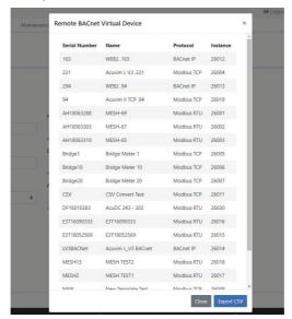
Figure 7-43 AcuLink 810 Remote BACnet Virtual Device List
