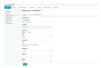
Figure 7-6 AcuLink 810 Modbus RTU Setting
