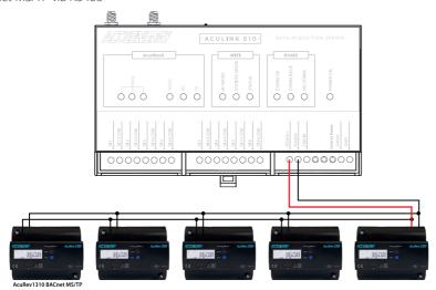
Figure 7-30 AcuLink 810 BACnet MS/TP via RS485 Protocol
