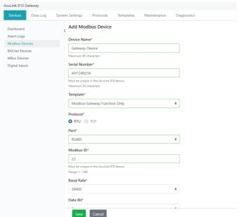
Figure 7-11 AcuLink 810 Modbus Gateway Function Setting
