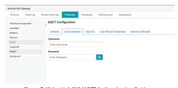
Figure 7-46 AcuLink 810 MQTT Authentication Setting
