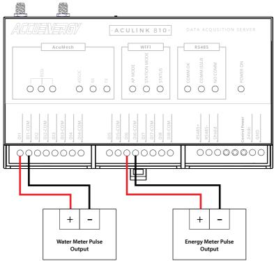
Figure 9-1 AcuLink 810 Digital Input Connections
