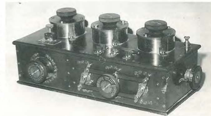
Photo 3. Multiple tuner from circa 1909 was used to tune receivers relying on magnetic detectors.
