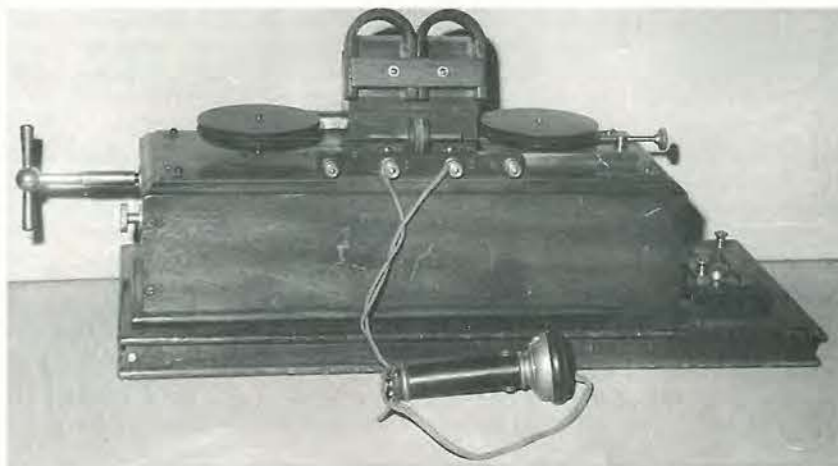
Photo 2. Marconi's magnetic detector, circa 1909, relied on the fact that electrical oscillations reduce magnetic hysteresis. The band around the wheels is iron wire, which passes between magnetic poles as the wheels rotate.
