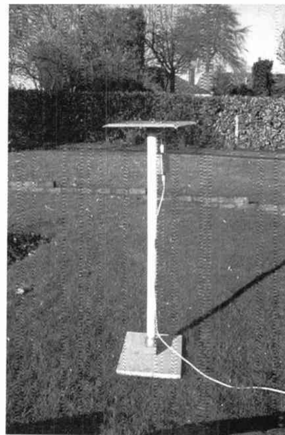
The author's prototype single-plate atmospheric detection platform.
