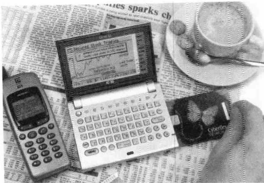
The Siemens IC35 Unifier provides Web access, E-mail and fax, it also includes a smartcard slot for future banking.
