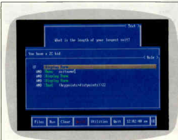
Crystal rule-building: The main window shows the rule currently being modified. Notice the English-like rule structure. The second window shows a form associated with the rule
