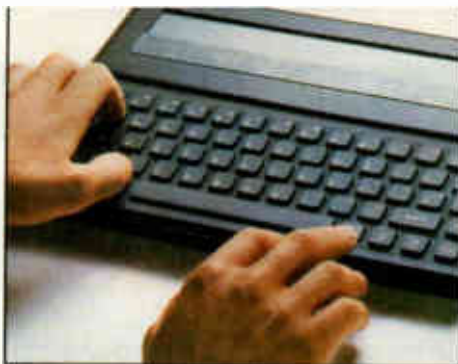
Full QWERTY keyboard offers 'silent', moving short-travel keys. Foldaway foot raises the Z88 12 1/2" for comfortable viewing and typing.
