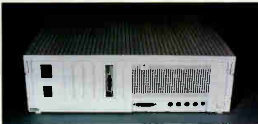
At the rear two 8-pin serial ports, handled by a Zilog 8530 controller, provide synchronous and asynchronous support for the Appletalk system
