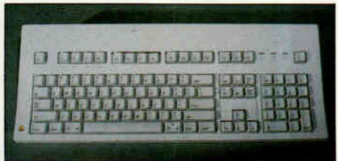
The Saratoga keyboard is larger and comprises 105 keys. These include 15 function keys — useful for IBM-style applications
