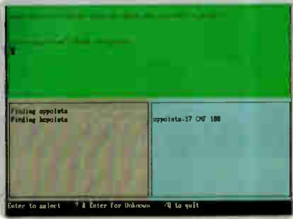
The VP-Expert bridge-bidding system in operation. The main window is for interaction with the user, while the other two provide information about the 'thinking' of the system
