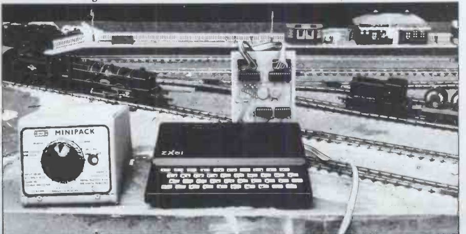
Proof that it can be done: a ZX81 controlling a model train set.
