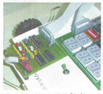
Interrupt-driven module connected to the PhizzyB input port.
