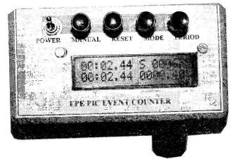
Front panel display window and function buttons; Mode 1 shown.
