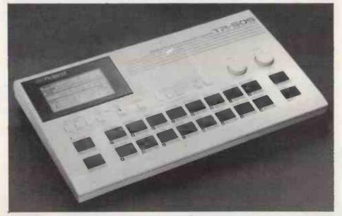
Your assumption is an erroneous one: only the TR505 and the RX21L have MIDI. The DDM220 only has Korg's 48ppqn sync standard, and so requires a synchronising device (like Korg's own KMS30) to work with MIDI machines.
