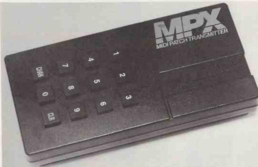
▶ New from Alesis is the MPX MIDI Transmitter, a hand-held remote control unit which allows you to send MIDI patch-changes to your MIDI equipment on any or all of 16 MIDI channels. Channel settings and patch numbers are entered from a numeric keypad on the MPX. As connection is via MIDI cable, it's possible to operate the MPX at quite a distance from your equipment – making the unit valuable both in the studio and on stage.
