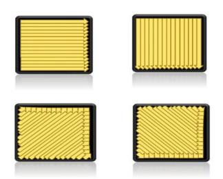
Fig. 5: Example of procedure for swab sampling, with black outline indicating the premarked area to be swabbed, yellow arrows indicating the direction for swiping. Swabbing starts as a) swab the marked area from left to right horizontally, b) swab the marked area from top to bottom vertically c) swab the marked area from bottom left to top right, and d) swab the marked area from top left to bottom right.
