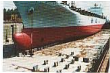
A ship with a small block coefficient and a large midship section coefficient
