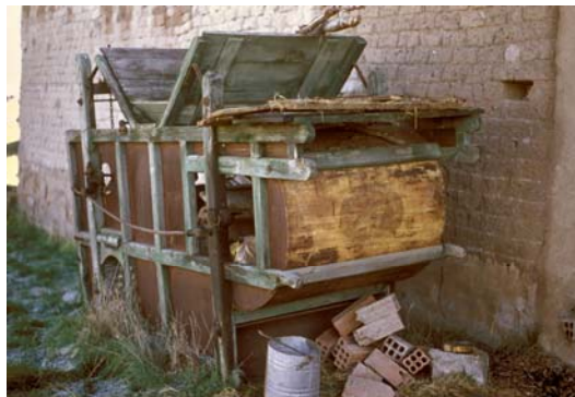
The winnower was used to separate the grain from the branch after it was threshed. It functioned with a motor. Photo provided by Federico Varona.
