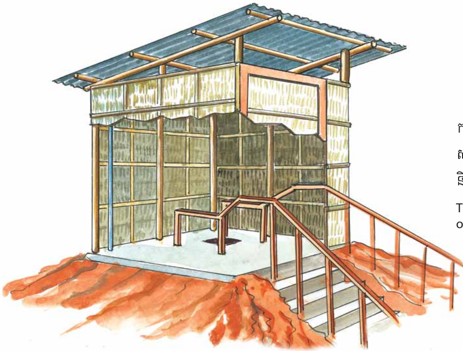
Figure 4: Superstructure for Latrine Equipped with Steps and Handrails.
