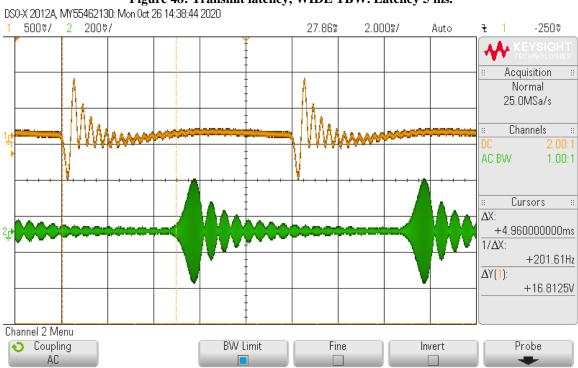
Figure 48: Transmit latency, WIDE TBW. Latency 5 ms.
