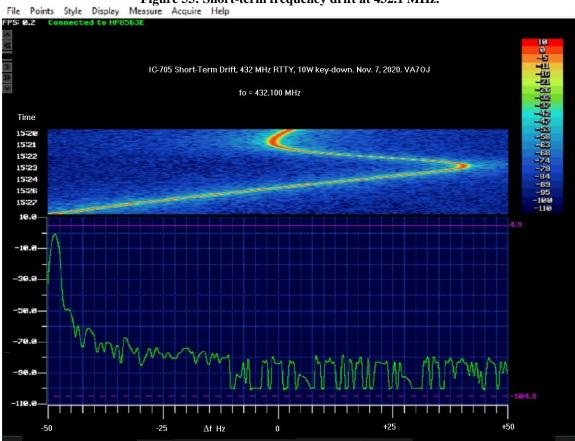
Figure 53: Short-term frequency drift at 432.1 MHz.
