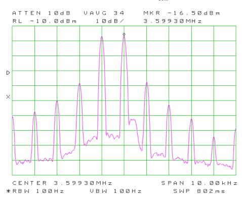
Figure 13: Spectral display of 2-tone IMD at 3.6 MHz, 10W PEP.
