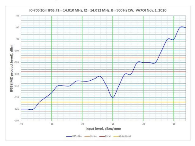
Figure 5: IFSS (2-tone IMD<sub>3</sub>) vs. test signal level.
