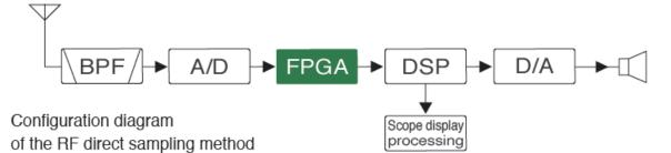
The FPGA also delivers a 1 MHz-wide digital video signal to the Scope Display Processing, which manages the screen displays, including the fast FFT spectrum scope, waterfall, audio scope and audio FFT (spectrum analyzer) as used in other Icom transceivers (7300 7610, 9700). The spectrum scope has a maximum span of  $\pm$ 500 kHz, adjustable reference level (-20 to 20 dB), video bandwidth and averaging, and minimum RBW  $\leq$  50 Hz.
