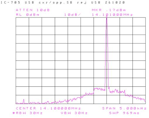
Figure 47: Carrier & opposite-sideband suppression at 14.1 MHz.
