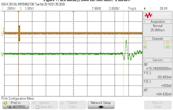
Figure 7: RX latency, 2400 Hz Soft filter. 2 ms/div.
