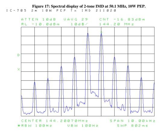
Figure 18: Spectral display of 2-tone IMD at 144.2 MHz, 10W PEP.
