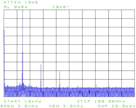
Figure 25. IC-705 20m Spurs/Harmonics 10W CW 211020
