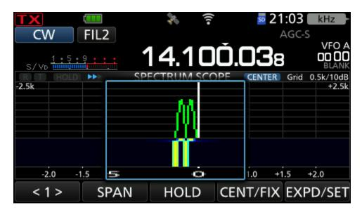
Figure 6a: Spectrum scope RBW (50 Hz).
