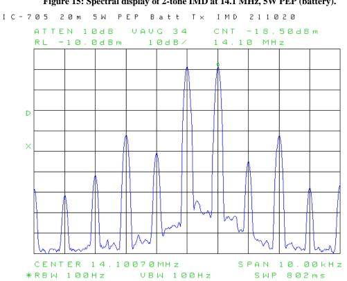
Figure 15: Spectral display of 2-tone IMD at 14.1 MHz, 5W PEP (battery).
