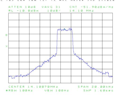
23: AM sidebands and THD with single-tone modulation. As in Test 26 above, the spectrum analyzer is connected to the IC-705 RF output via a 50 dB high-power attenuator. On the IC-705, RF Power is adjusted for 2.5W resting carrier.  $A \pm 1$  kHz test tone is applied to the USB port from the tone-generator program running on the laptop computer. The spectrum analyzer records the carrier and sideband parameters.
