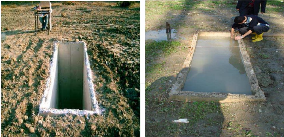
Figure 6.11: Trench barriers, after (Flrat et al. 2010).
