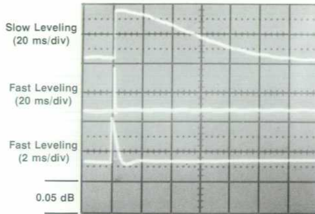
Fig. 4. Slow and fast leveling loop responses to an output short-to-open transition.
