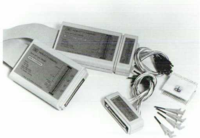
Fig. 4. The versatile probing scheme for the 1611A Opt 001 permits a variety of methods for connecting the analyzer to the unit to be tested.
