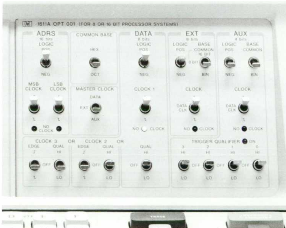
Fig. 2. Front panel of the general-purpose module for the 1611A Logic State Analyzer. Seven clock inputs enable information on several buses to be captured for simultaneous display.
