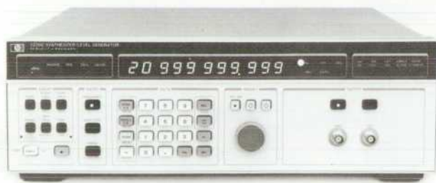
Fig. 1. Model 3336A/B/C Synthesizer/Level Generator (3336C shown) generates precise frequencies and levels over a frequency range of 10 Hz to 20.999 999 999 MHz. Output levels are accurate within \pm 0.05 dB, and integrated phase noise is less than -60 dBc.
