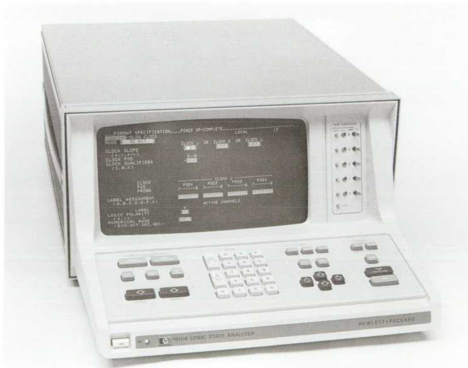
Fig. 1. Model 1610B Logic State Analyzer features multiphase clocking. Three clock inputs, each with four qualifiers, may be used to capture events in a digital system that do not occur simultaneously. A major application is decoding multiplexed buses.
