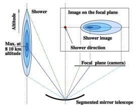
Imaging of a γ-ray initiated e.m. shower by a telescope. Image taken from Völk and Bernlöhr (2009)
