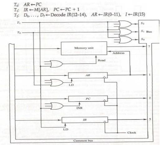
Figure 5-8 Register transfers for the fetch phase.
