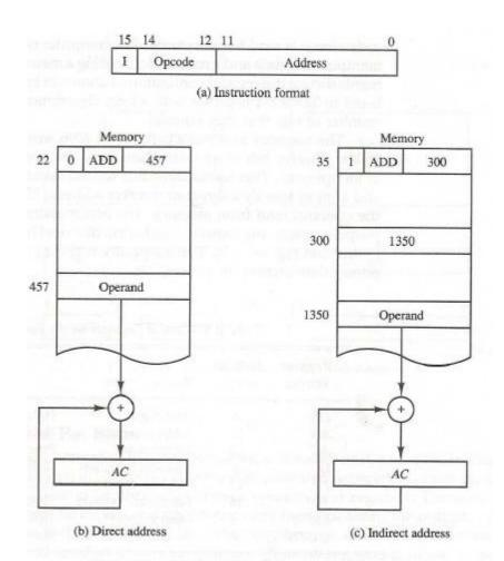
Figure 5-2 Demonstration of direct and indirect address.
