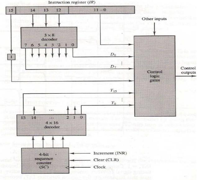
Figure 5-6 Control unit of basic computer.
