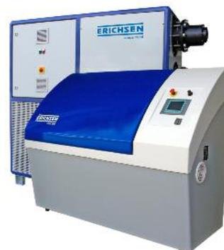
*Corrosion tester for salt spray and cyclic climate tests with controlled humidity. Constant, increasing- and decreasing ramps for temperature and humidity are programmed via "Touch" display. With an additional air conditioning unit, low-temperature cycles up to -40 °C can be performed.*
