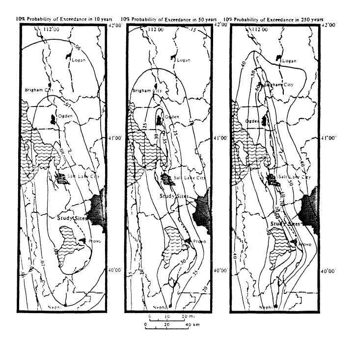
Figure 3. Contours of peak ground acceleration on soil sites with 10 percent probability of being exceeded in 10 years. 50 years and 250 years. Peak accelerations on rock sites are expected to be approximately 10 percent higher than the values shown on the map for 10 percent probability of exceedance in 10 years and approximately 20 percent higher than the values shown on the maps for 50 and 250 years (modified from Youngs and others, 1987).
