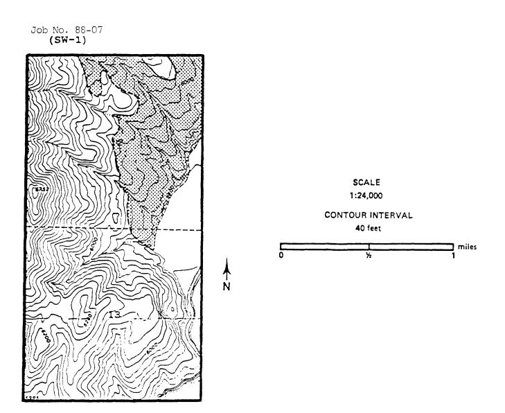
Figure 4. Potentially suitable area (\*\*\*\*) for a landfill in sections 12&13, conditions are variable and stratigraphic investigations are required to demonstrate site suitability and to provide information for site design and construction.
