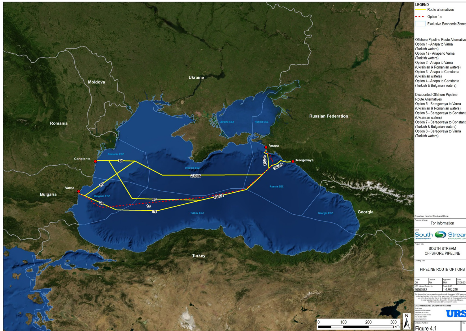
Figure 4.1: Pipeline Route Options
