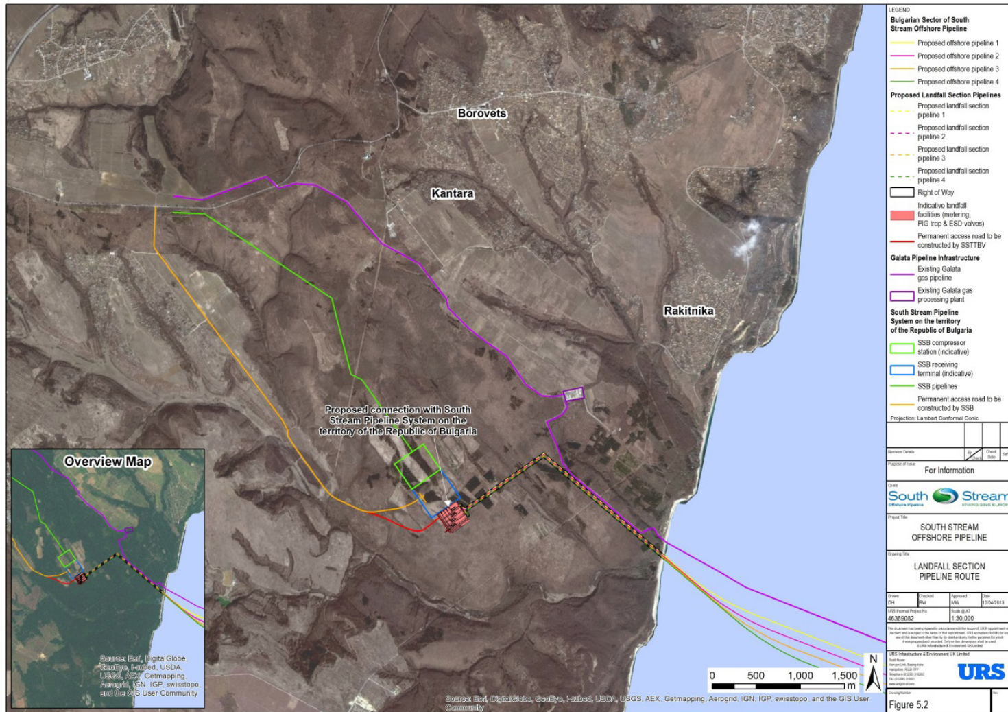
Figure 1.12: Landfall section of the Bulgarian Sector of the South Stream Offshore Natural Gas Pipeline
