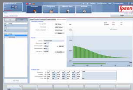
Fig 5: Example of a simulated test run conducted using Carb-o-Prof software.
