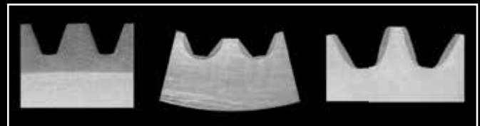
Hardness Pattern on Cut Samples
