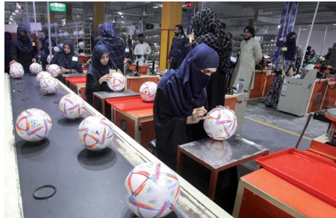
Workers conduct the final check to fix any cavity in the seams of balls inside a soccer ball factory in Sialkot, Pakistan, on December 2, 2022. (REUTERS)
