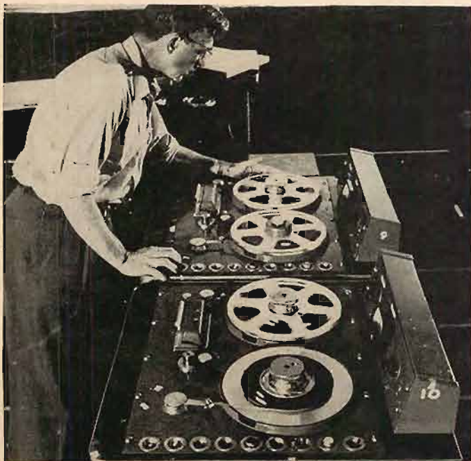
Fig. 7. RCA Victor's first two-track stereo recorders, Model RT-11, with "home-made" two-track in-line heads for 1/4-in. tape. These were used in 1954 to record "Zarathustra" performed by Chicago Symphony Orchestra, Fritz Reiner conducting. (Photo courtesy Bill Miltenburg.)
