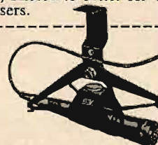
ALTEC 685A CARDIOID MICROPHONE SHOWN IN ALTEC 191A BOOM MOUNT Frequency Response: 40 to 16,000 cycles • Output Impedance: 30/50, 150/250, 20,000 ohms • Output Level: -54 dbm/10 dynes/cm 2 • Discrimination: Average front-to-back, 20 db • Hum: -120 db (Ref.: 10 -3 Gauss) Price $96.00 net
