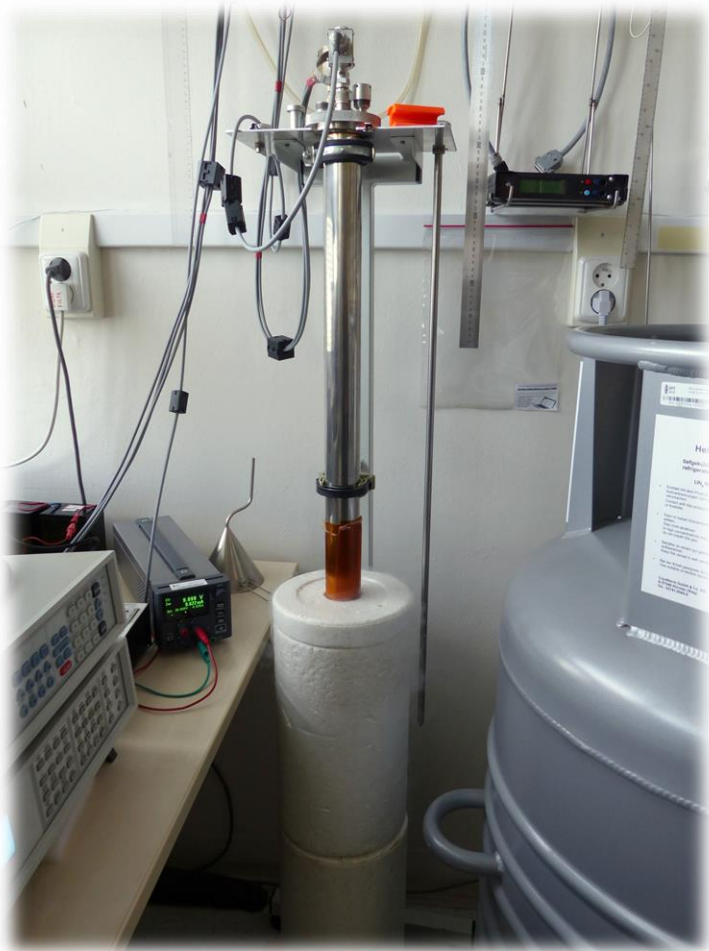
Sample pre-cooled with liquid nitrogen
