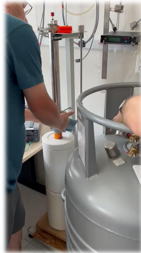
Evacuation and placing Emister into Dewar vessel
