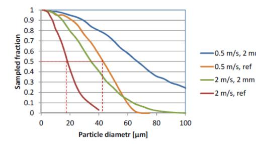
Particle collection efficiency obtained using reverse sampling according to flue gas velocity in the duct (0.5 m/s and 2 m/s) and nozzle diameter (ref stands for 8 mm nozzle diameter) at a sample rate of 10 l<sub>sto</sub>/min
