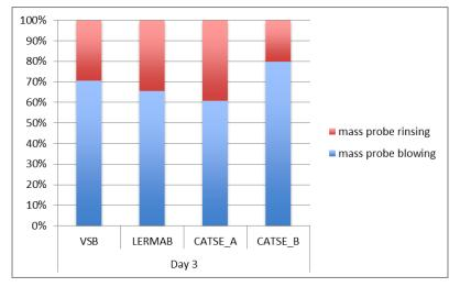
Contribution of deposit in the probe determined by rinsing and blowing. More than 60% of the total deposits are removed by blowing.
