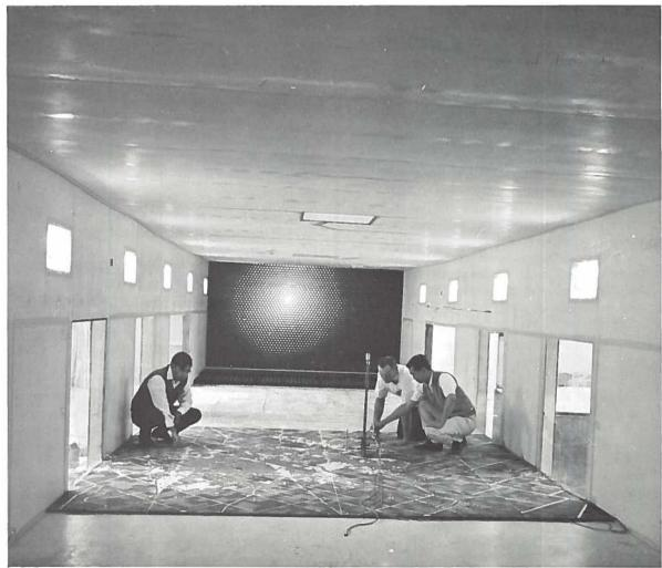
Model of Fort Wayne, Indiana, prepared for wind and contaminant concentration measurements in the new environmental wind tunnel of the Fluid Dynamics and Diffusion Laboratory (1:4000 horizontal scale; 1:2000 vertical scale).
