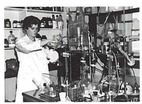
Laboratory technician determining inorganic nitrogen content of the soil samples, San Luis Valley Branch Experiment Station, Center, Colorado.
