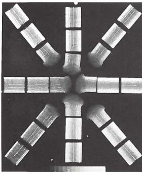
Density gradients in particleboard shown by X-ray absorption patterns.
