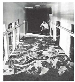
Model of Eagle River Valley-Climax region in low-speed wind tunnel (1:9600 scale).
