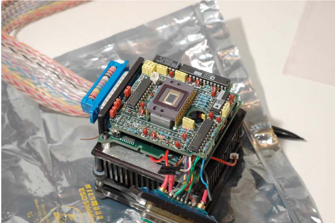
Figure 2 : An assembled camera without the housing case. Clearly seen is the upper board with the CCD sensor (KAF 0402ME) inserted. Below it is the lower board and below that the cooling assembly including the peltier cooler (not seen) and the fan assembly.
