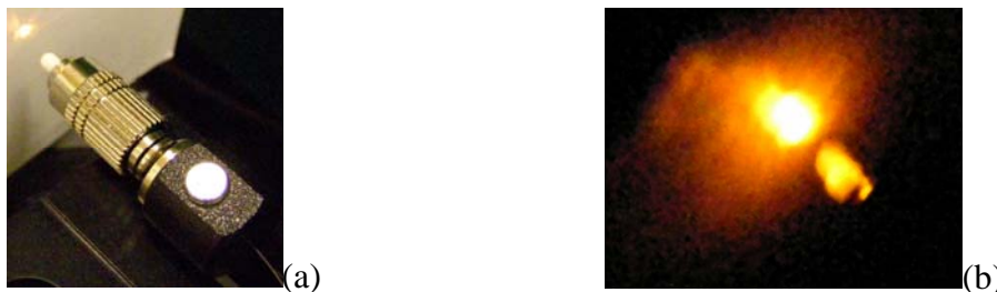
Fig.3 The supercontinuum shown on a screen; when the PCF was pumped with 775 nm, 200 fs pulses at (a) 10 mW; and (b) 50 mW.
