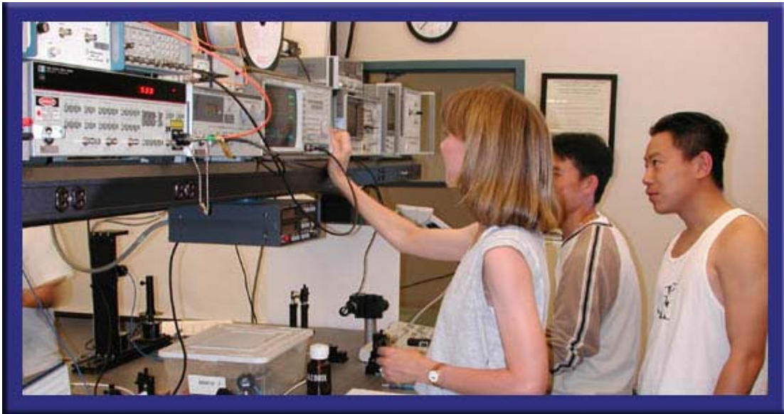
Figure 1: Undergraduate photonics teaching laboratory station. This is one of three identical benches used in two of our undergraduate laboratory courses. The room is 600 square feet. It also accommodates a photonics research bench. In this particular exercise the students are measuring the modal dispersion-limited bandwidth of a multimode optical fiber at 850nm.
