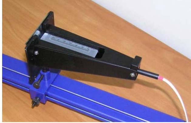
Fig. 4. Focal monochromator on a base of holographic lens.
