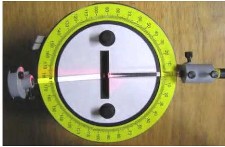
Fig. 15. Fiber loss studying while misalignment of models of fiber optics elements.
