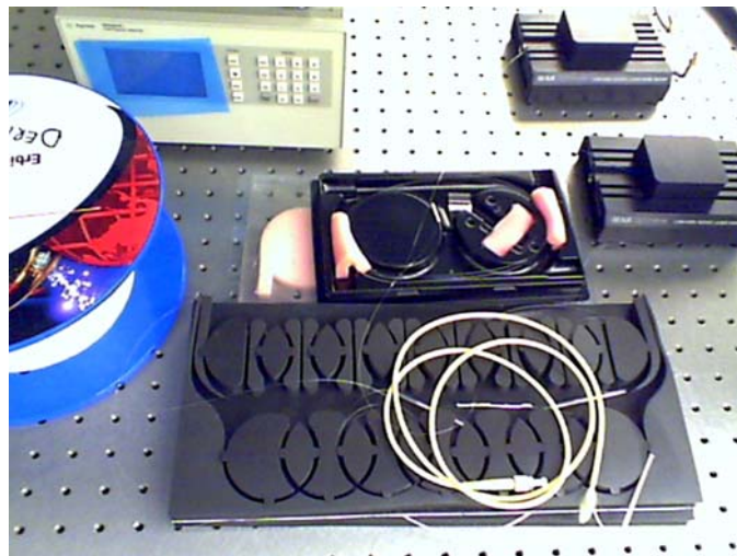
Figure 2: The Erbium-doped fiber amplifier assembly used in the EE443 fiber optic communication lab is shown. The students adjust the bias conditions of the pump laser. Experimental measurements on the amplifier are compared to computer simulations.
