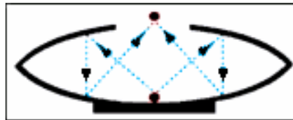
Fig. 2. Ray paths between parabolic mirrors [1].
