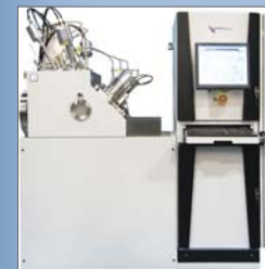
Voyager enables diamond-like carbon coatings over large, 3D components.
