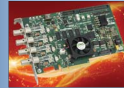
FireBird CoaXPress frame grabber with four 6 Gbps (CXP-6) links.
