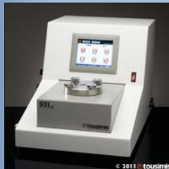
The tousimis® 931 is a programmable multi-application critical point dryer.
