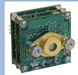
Eye-safe, high-performance, feature rich APD-based laser rangefinder receiver module.
