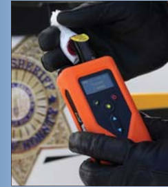
DeltaNu's ReporteR is a handheld Raman Spectrometer used for material identification.
