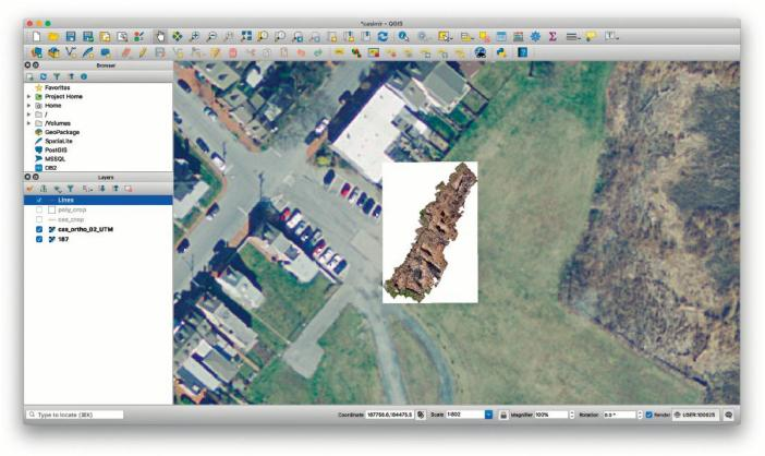
FIGURE 2. GIS combining aerial photography and an orthomosaic map of the excavations from photogrammetry.
