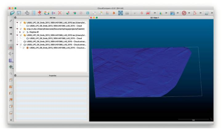
FIGURE 4. Bare-earth mesh derived from LiDAR point cloud.
