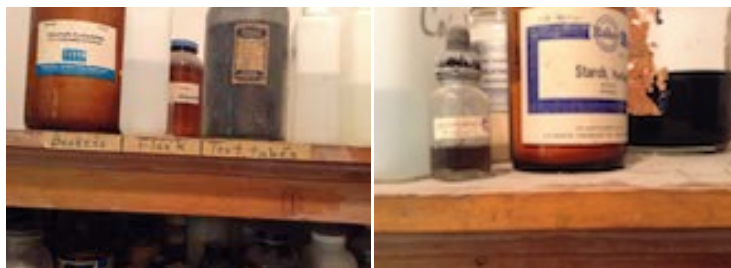
Figure 2. Middle school prep/storeroom hazardous areas. An “un-lipped” top shelf storage above eye level with old chemicals in eroding containers.
