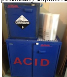
Acid cabinets not locked nor vented.
