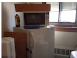
Chemical refrigerator not labeled. NO FOOD sign missing.
