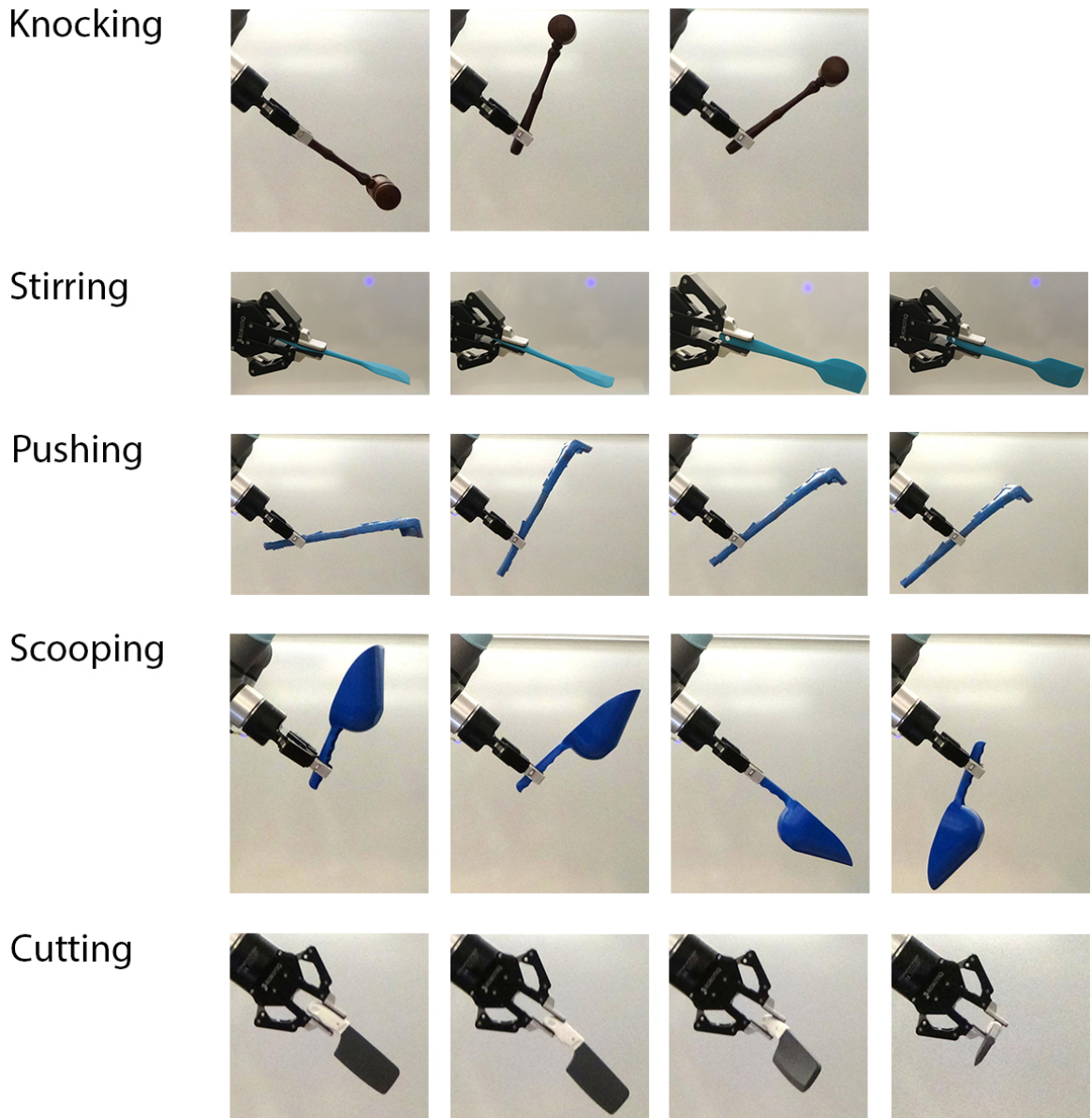
Figure 3.6: Different grasping poses of the source tools (Star 1). For each task, that is, knocking, stirring, pushing, scooping, and cutting, at least three different grasping poses were tested.
