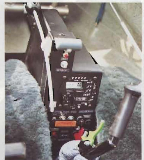
The lower panel with the Ilec engine control instrument
