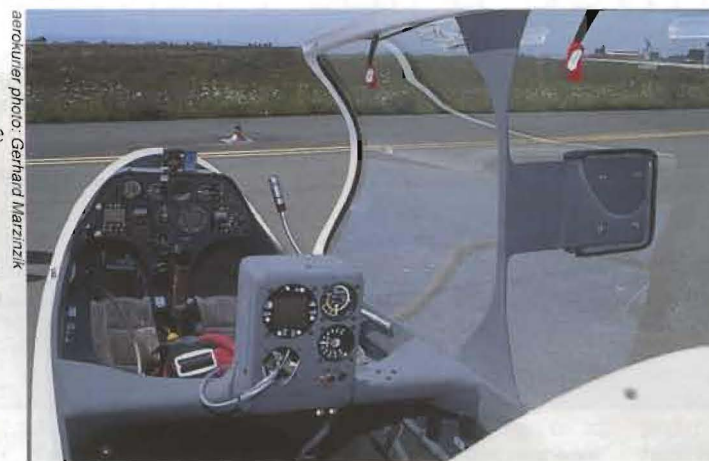
The bespoke cockpit means that a tiny panel can be used in the rear to aid visibility
