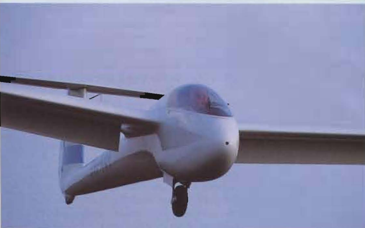
The first glass-fibre sailplane: the Akaflieg FS-24 Phoenix, one of eight built. The type's maiden flight was in 1957. It has a max L/D of 40 and a 16m wingspan
