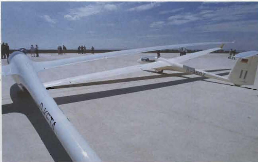
A 15-metre span glider fits comfortably under one wing of D-KETA – whose span is 30.9m/101.38ft
