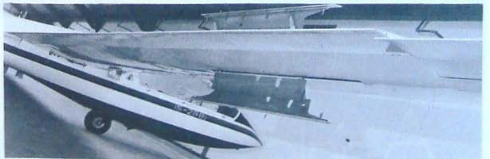
Large top and bottom surface airbrakes, with flaps give good landing characteristics.
