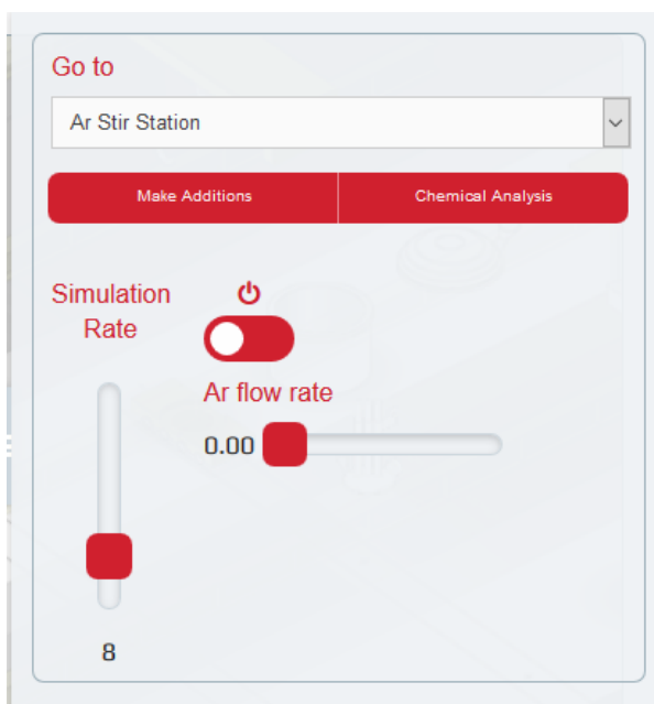
Figure 8-6. Screenshot of control panel of Ar Stir Station.
