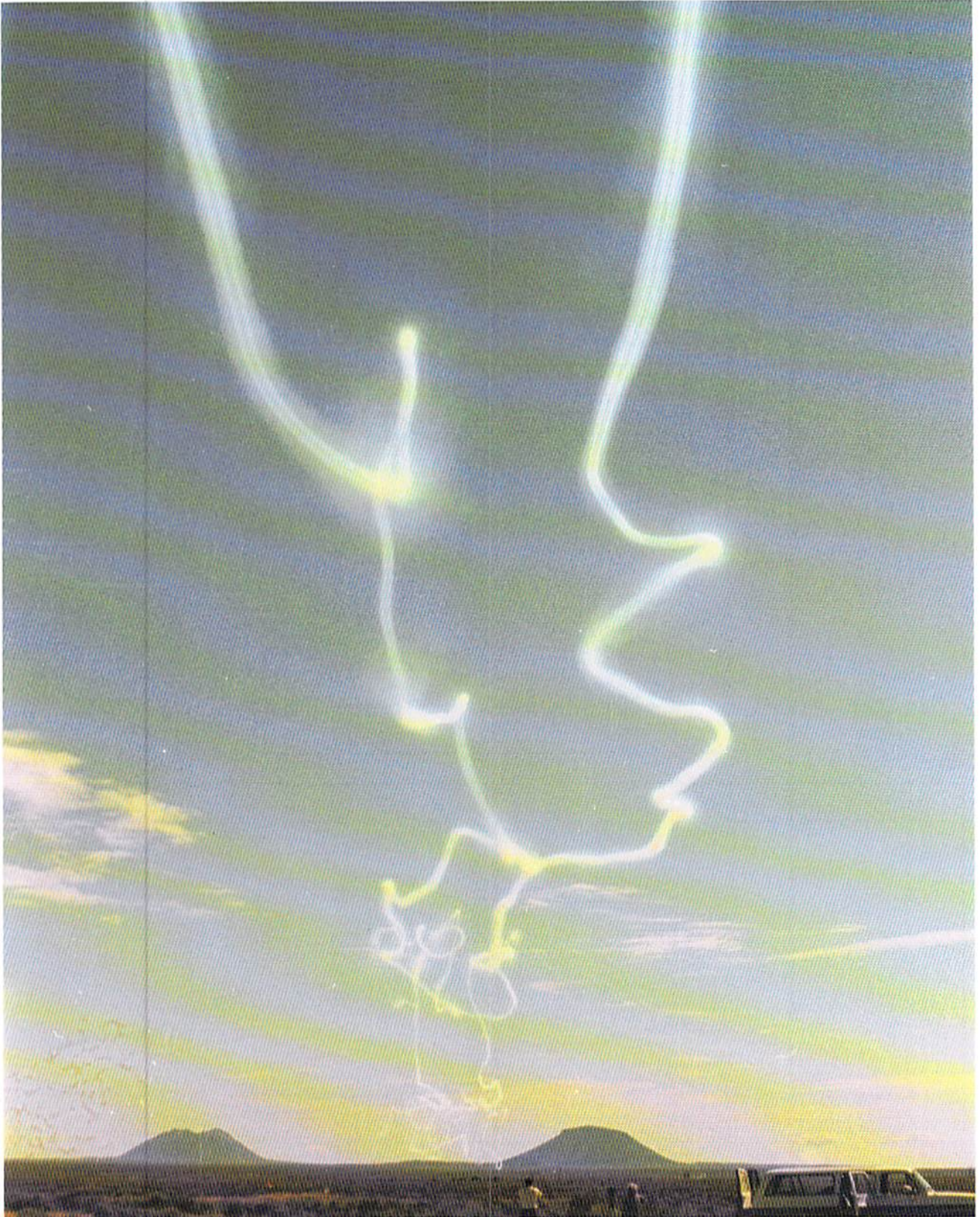
Figure 6. B-727-222 airplane visualized trailing vortex system showing extreme sinusoidal instability.
