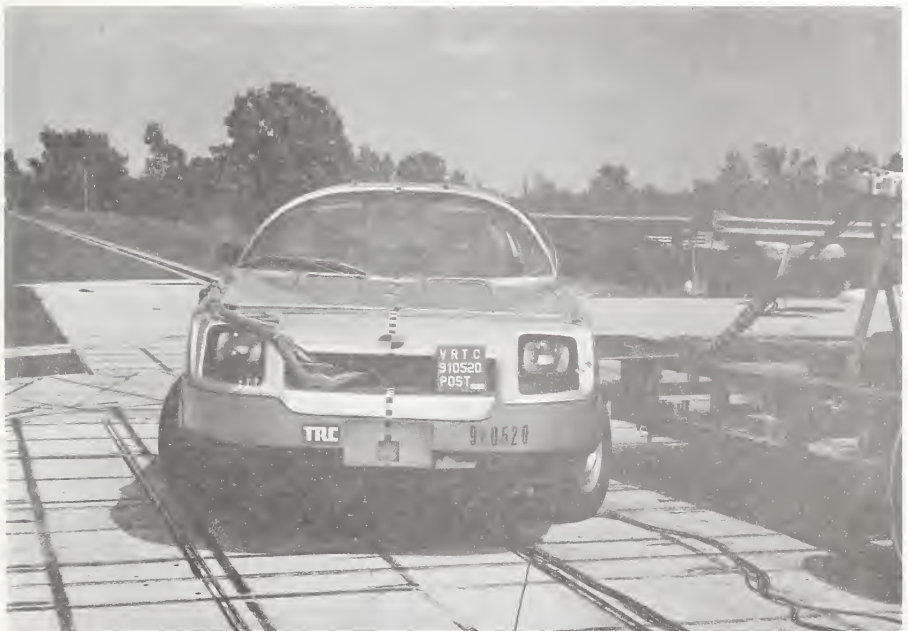
Figure A-2. POST-TEST VEHICLE FRONT AND BARRIER VIEW
