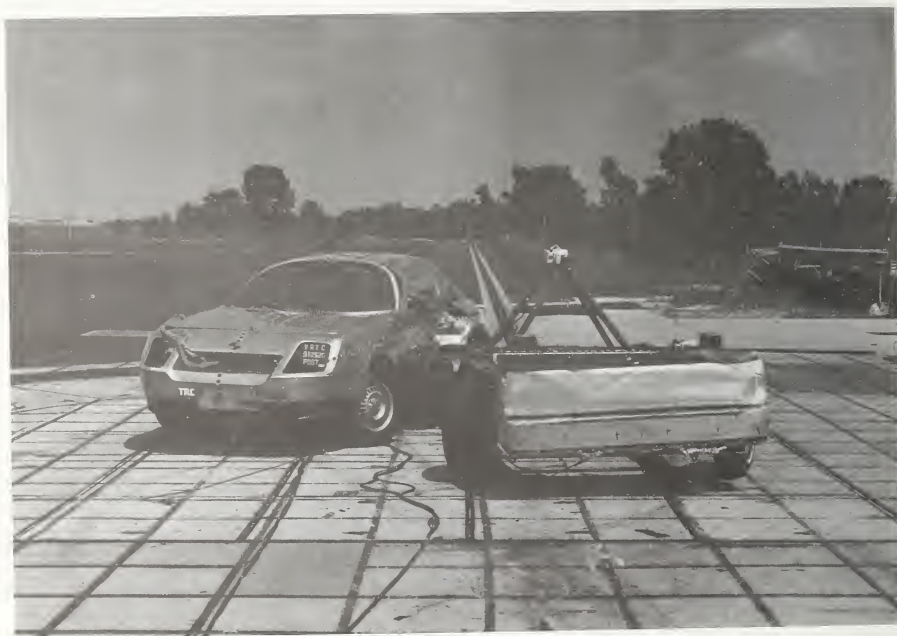
Figure A-16. POST-TEST VEHICLE LEFT FRONT AND BARRIER VIEW
