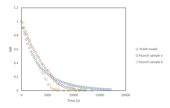
Figure 9-6. A non-linear regression was used to find the optimum D value for the set conditions, this gave D = -0.714 in the Hukill equation producing an R<sup>2</sup> of 0.928.
