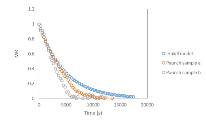
Figure 9-5. Comparison of Hukill model for 1 x 10<sup>-11</sup> m depth to paunch thin layer 35 °C, 40% RH samples a and b.
