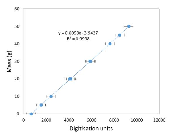
Figure 4-3. Calibration mass versus digitisation units from the load cell and data logger system.
