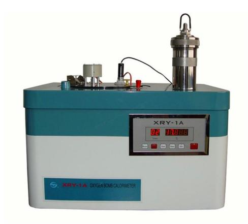
Figure 6-1. An XRY-1A Oxygen Bomb Calorimeter (Nanbei 2014).
