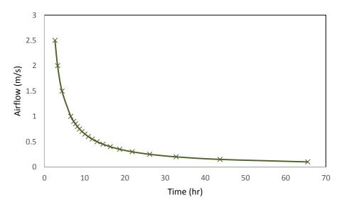
Figure 8-8-3. Airflow (m/s) versus time (hours). An increase in airflow from approximately 1 m/s does not greatly improve drying rates.
