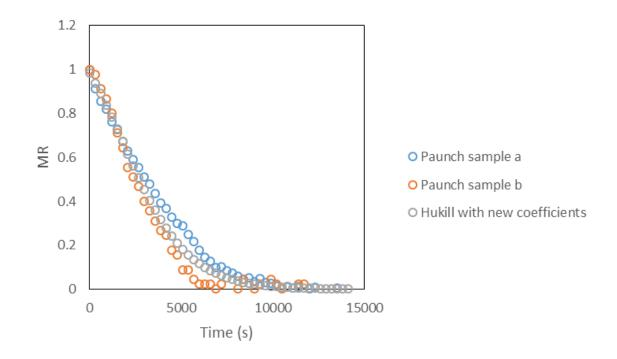
Figure 9-8. The Hukill equation with coefficients added to the time constant, R<sup>2</sup> values are 0.997 for the thin layer and 0.998 for the 2.5 cm sample.
