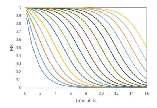
Figure 9-1. The standard deep bed drying curves from the Hukill equation.
