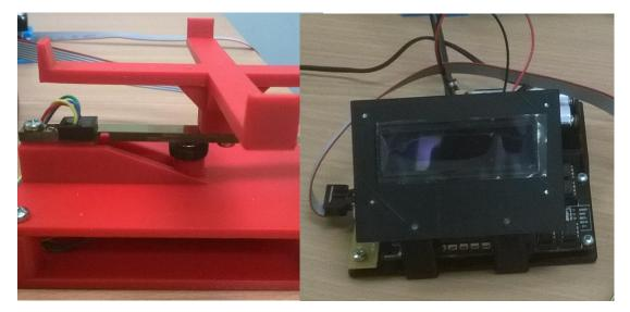
Figure 3 - Load cell incorporated into a tray holder (left) which is wired into the data logger (right)
