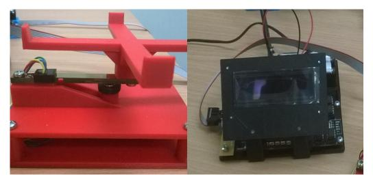
Figure 4-1. A 50 gram load cell and tray holder (left) wired into a custom built data logger (using a Picaxe microcontroller) (right).
