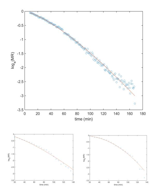
Figure 4-8. Page equation fit for 35 °C, 40% relative humidity thin layer grain type sample (top) and two grass type samples (bottom).
