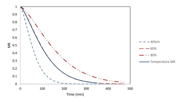
Figure 9-3. MR versus time (min) for MR (40, 60, 80% RH) and MR (35, 45, 55°C).
