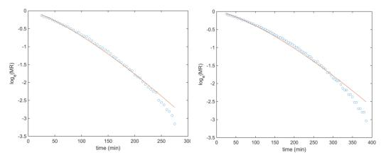
Figure 4-10. Page equation fit for 35  $^\circ C,$  60% relative humidity thin layer grain type samples.
