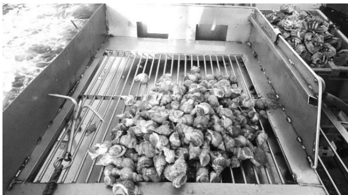
Figure 7.1. The whelk riddle used on Vagabond DO180 in the Isle of Man.
