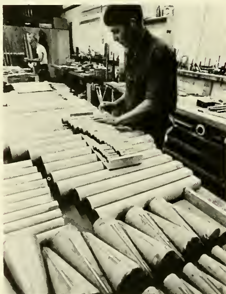
Steve Boody transfers pipe measurements with proportional dividers. In the foreground are conical feet of pipes; cylindrical parts are pipe bodies.
