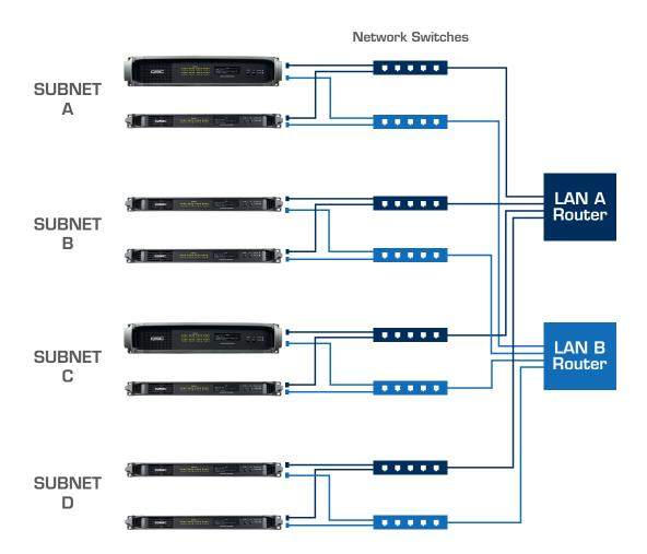
In the above example, consider four redundant subnets with a router for each of "LAN A" and "LAN B". Each subnet will have an IP gateway through which traffic to other subnets will be forwarded. The appropriate gateway entries are added to each unit's Ethernet settings in Q-SYS Configurator.
