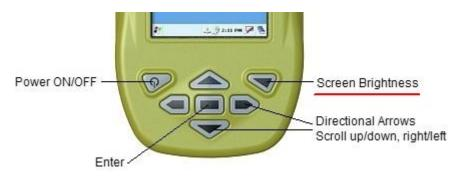
Figure 2-5 MEZ1500 Keypad - Screen Brightness Button.
