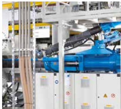
The compounded melt flows directly from the single-screw extruder to the plasticizing unit of the injection molding machine.
