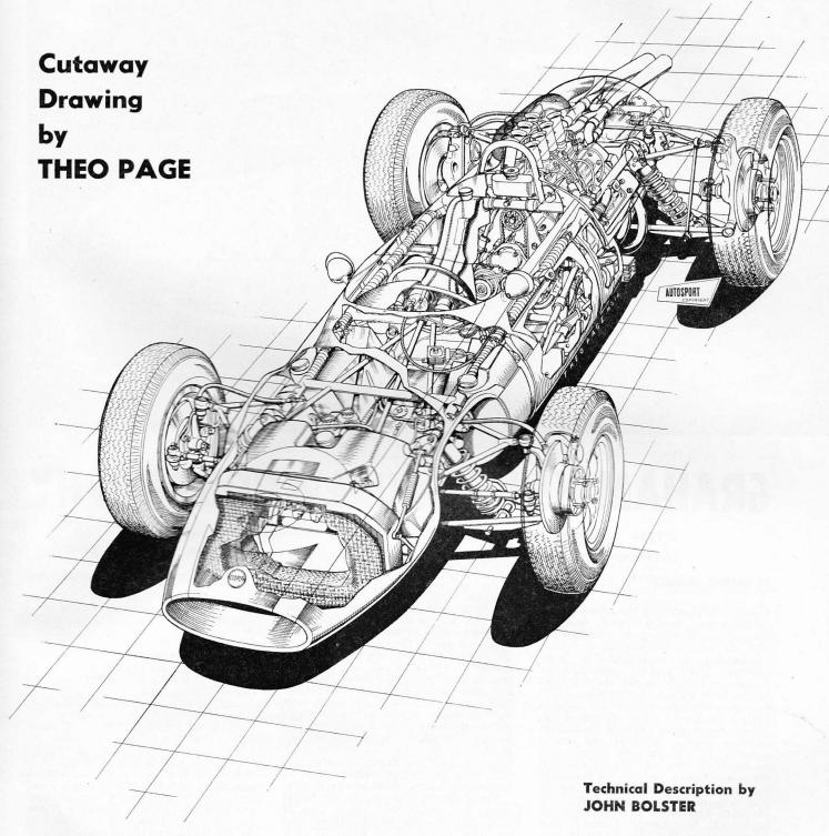
$T^{\text{HE}}$  new Cooper does not differ greatly from last year's model. It is narrower and lower and has been "cleaned up", but most of the well-tried Cooper features are retained.
