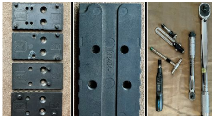
Figure 2 – L-R: Close-up of GLOCK® MOS plates showing the holes and bosses, upside-down MOS plate, torque screwdrivers, and torque wrenches.
