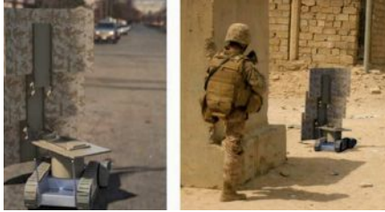
Lightweight composite materials mounted onto autonomous ground vehicles
