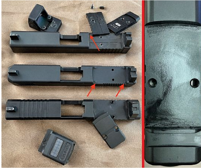
Figure 1 – Left side: OEM GLOCK® MOS slide with OEM and aftermarket plates. Below that are two aftermarket slides for a GLOCK 19 Gen3; Right side: A badly machined slide which has no bosses needed to take the G forces. (photo courtesy of Christopher Galli)
