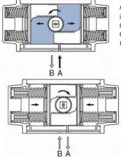
Air supplied to Port A forces pistons apart and toward end position, compressing springs. Exhaust air exits at Port B. (A counter-clockwise rotation is obtained)
