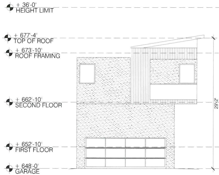
UNIT 1 - WEST EXTERIOR ELEVATION ③
