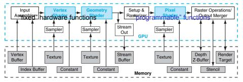
Various objects and buffers are allocated in the GPU memory hierarchy
