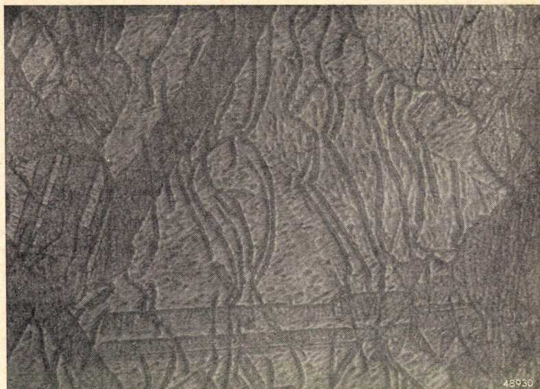
Fig. 13. Ag with 0.58 % Mg, 40 h. 650° air (+6½ h. 800° air); etched NH_4OH + H_2O_2 . Magn. 600 ×. Inner oxide films, running roughly parallel to the surface of the strip. Arrow indicates direction of penetration of O.
