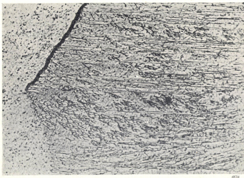
Fig. 9. Same specimen as of fig. 8. Magn. 1000×. Inner oxide film forming part of the oxidation boundary. The depth of oxidation close beside the oxide film appears to have profited from the oxygen barred by it. Arrow indicates direction of penetration of O.
