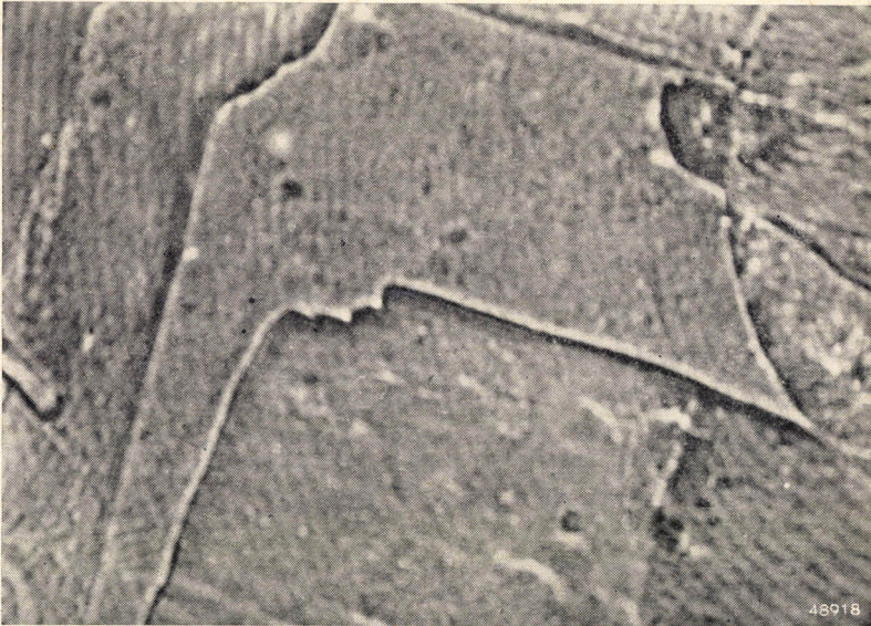
Fig. 17. Round rod of Cu with 0.25 % Be, oxidized in air at 950 °C in relay-controlled furnace. Deep etch with \text{HNO}_3 . Magn. 150 \times . Up to the oxidation boundary (inner circle) vague rings are visible, suggesting a Liesegang phenomenon, but caused by the temperature oscillations.
