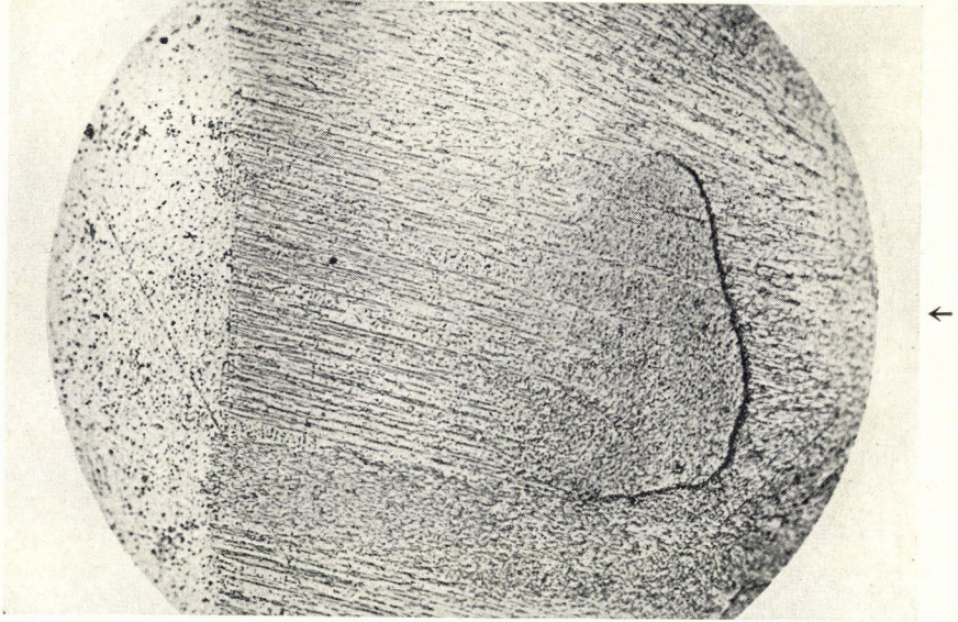
Fig. 10. Same specimen as figs 8 and 9. Magn. 500×. Inner oxide film "behind the front". Arrow indicates direction of penetration of O.
