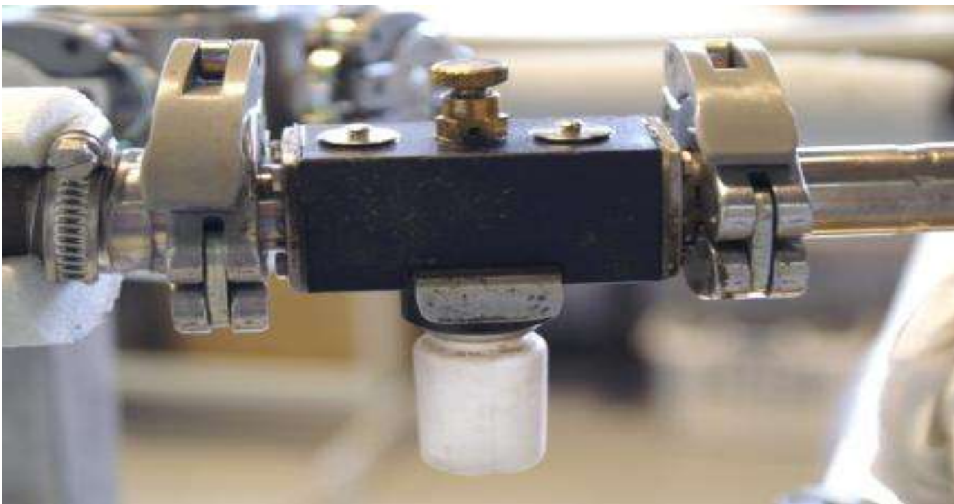
Fig. 7.8. Prototype sampling device. 10 increments each of 10 ml were sampled during a period of 10 minutes – an effective composite sample for chemical reference analysis. (Holm-Nielsen et al. 2007)
